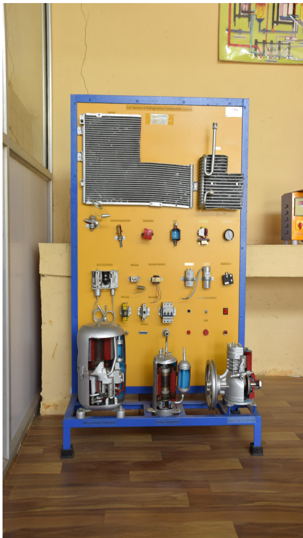
Cut section of refrigeration trainer
